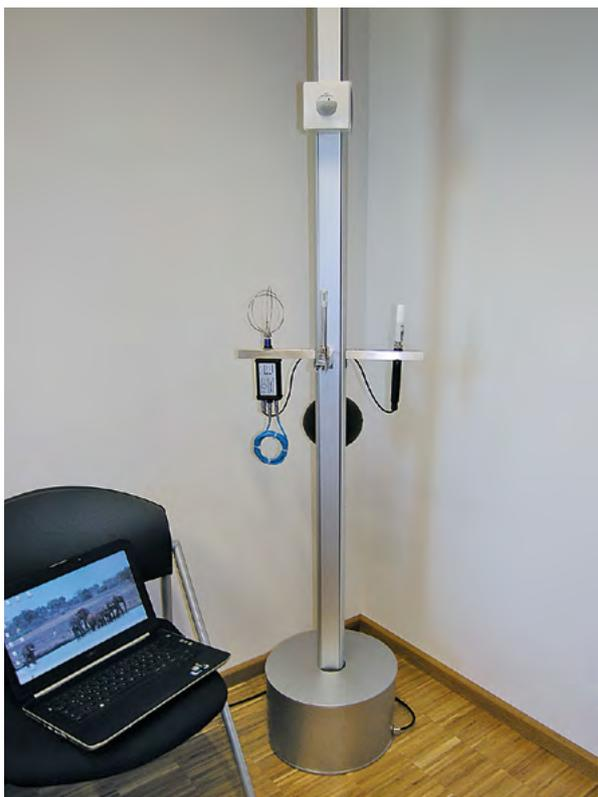
Measuring carbon levels to verify ventilation concepts
