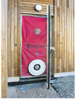
Measuring the airtightness of the Federal Environment Agency's Haus 2019 building with the differential pressure measurement method
