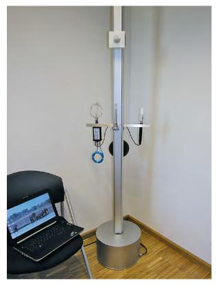
Measuring carbon levels to verify ventilation concepts
