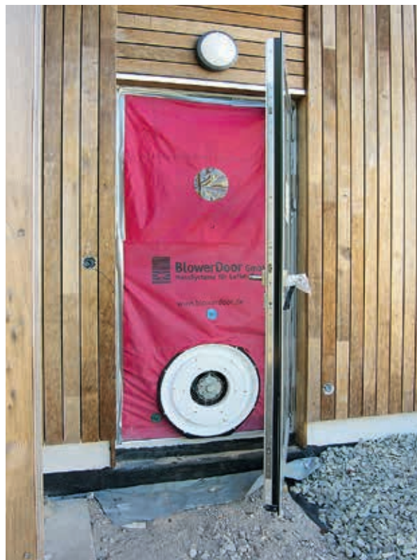
Measuring the airtightness of the Federal Environment Agency's Haus 2019 building with the differential pressure measurement method
