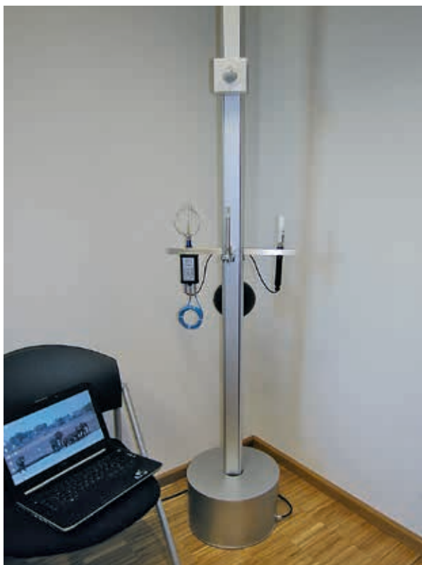
Measuring carbon levels to verify ventilation concepts
