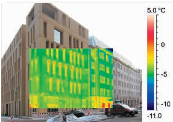
Thermographic testing of the street-side facade of the old and new BMU building in Berlin in order to check the quality of construction
