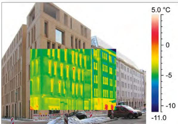
Thermographic testing of the street-side facade of the old and new BMUB building in Berlin in order to check the quality of construction
