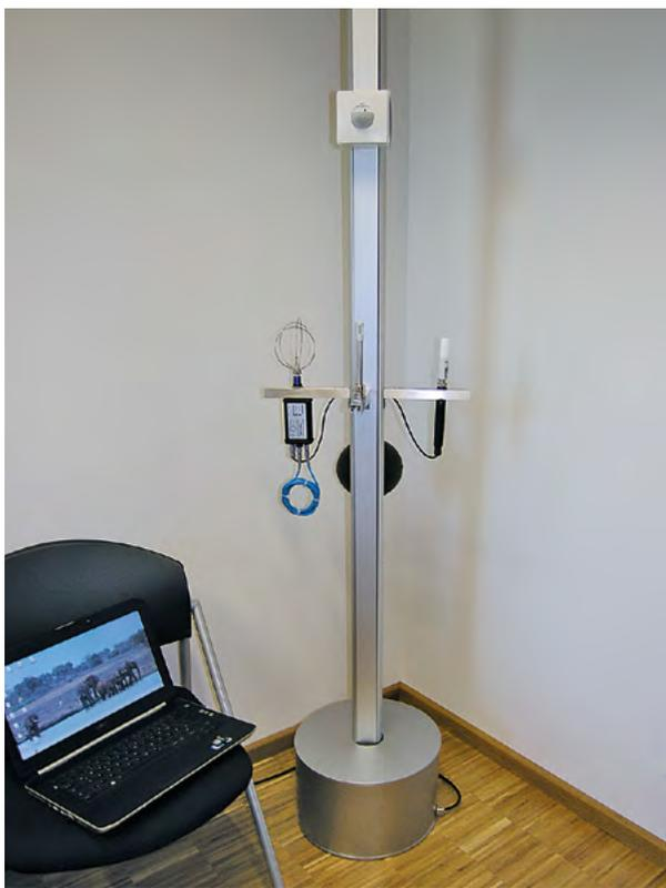
Measuring carbon levels to verify ventilation concepts
