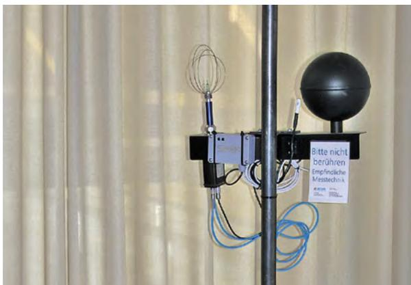
Determining and verifying interior comfort parameters during the operating phase
